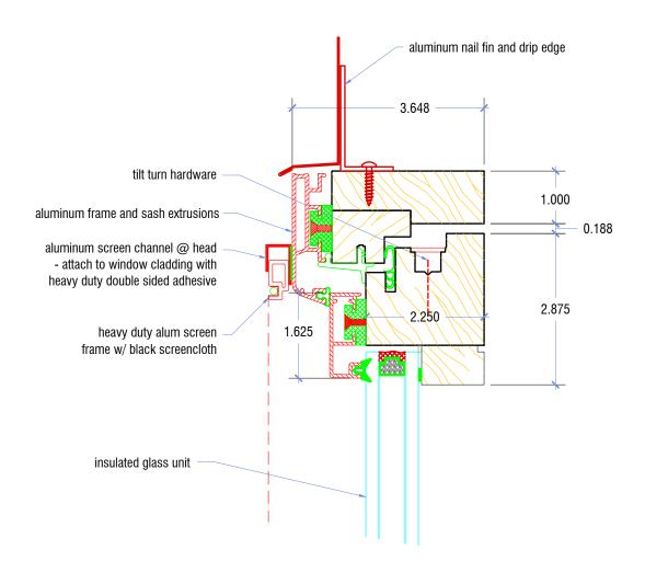
1.75" ALUMINUM CLAD INSWING CASEMENT W/ SCREEN AT HEAD
